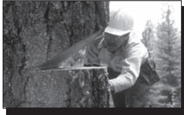
Figure 4-23—The sloping cut is a 45-degree angle.
