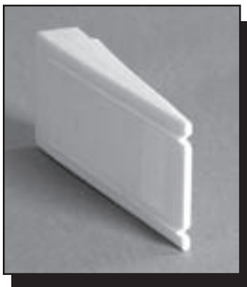
Figure 5-12—A rifled single-taper wedge is designed to provide lift when a tree is felled. It can be stacked with additional rifled single-taper wedges. The rifling helps keep the wedges aligned and stacked as they are being driven.
