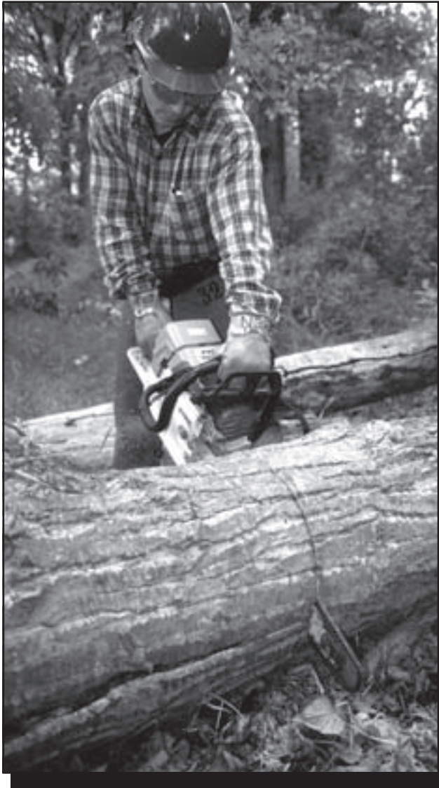
Figure 4-11—Watch the kerf for movement that will indicate a bottom bind (kerf opens) or top bind (kerf closes).
